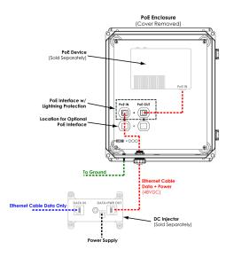
14x12x07 Fiberglass Reinf Polyester FRP Weatherproof Outdoor IP24 NEMA 3R Enclosure, PoE MNT PLT, Solid State Thermostat 48 VDC Fan Gray from Lcom has same day shipment for domestic and International orders. Our portfolio includes coaxial cable assemblies, connectors, adapters and custom products as well as lightning and surge protectors, NEMA rated enclosures, and an RF product line which includes antennas, amplifiers, passive, and active components.
