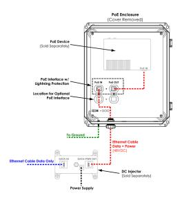
18x16x08 Fiberglass Polyester FRP Weatherproof Outdoor IP24 NEMA 3R Enclosure, 802.3af PoE MNT PLT, Solid State Thermostat 48 VDC Fan Gray from L-com has same day shipment for domestic and International orders. Our portfolio includes coaxial cable assemblies, connectors, adapters and custom products as well as lightning and surge protectors, NEMA rated enclosures, and an RF product line which includes antennas, amplifiers, passive, and active components.
